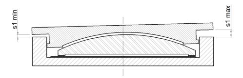
The report of the bearing inspection must be performed according to the EN1337-10 Annex B and the data recorded in the "Bearings inspection report" (see the following pages).
